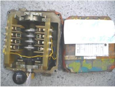
A photograph of a yellow combination switch assembly with its cover removed, showing internal components that appear disorganized and possibly damaged.         |
