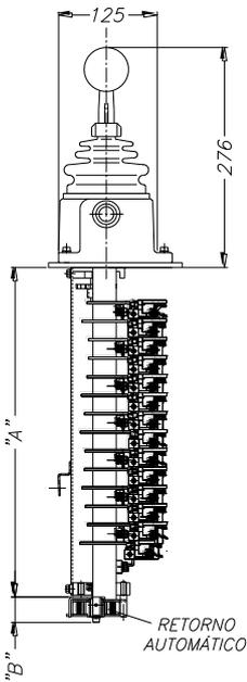
CHAVE SEM CAIXA PARA MONTAGEM EM CONSOLE COM SENSORES
