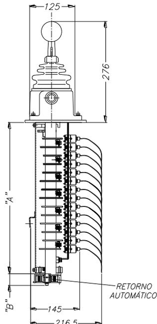
CHAVE SEM CAIXA PARA MONTAGEM EM CONSOLE COM SENSOR E POTENCIÔMETRO
